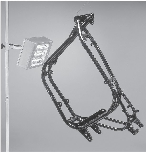
Example of Curing a Motorcycle Frame
