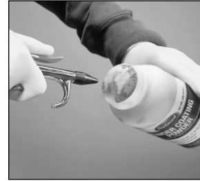
Blow remaining powder out of bottle with air hose
