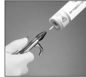
Direct air down nozzle to remove powder
