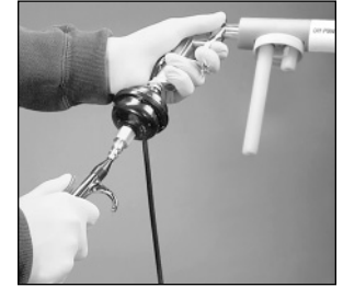
Press trigger and blow remaining powder out of the discharge tube
