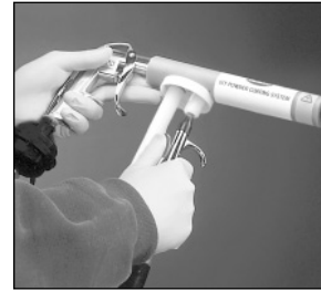
Blow remaining powder out of pick-up tube
