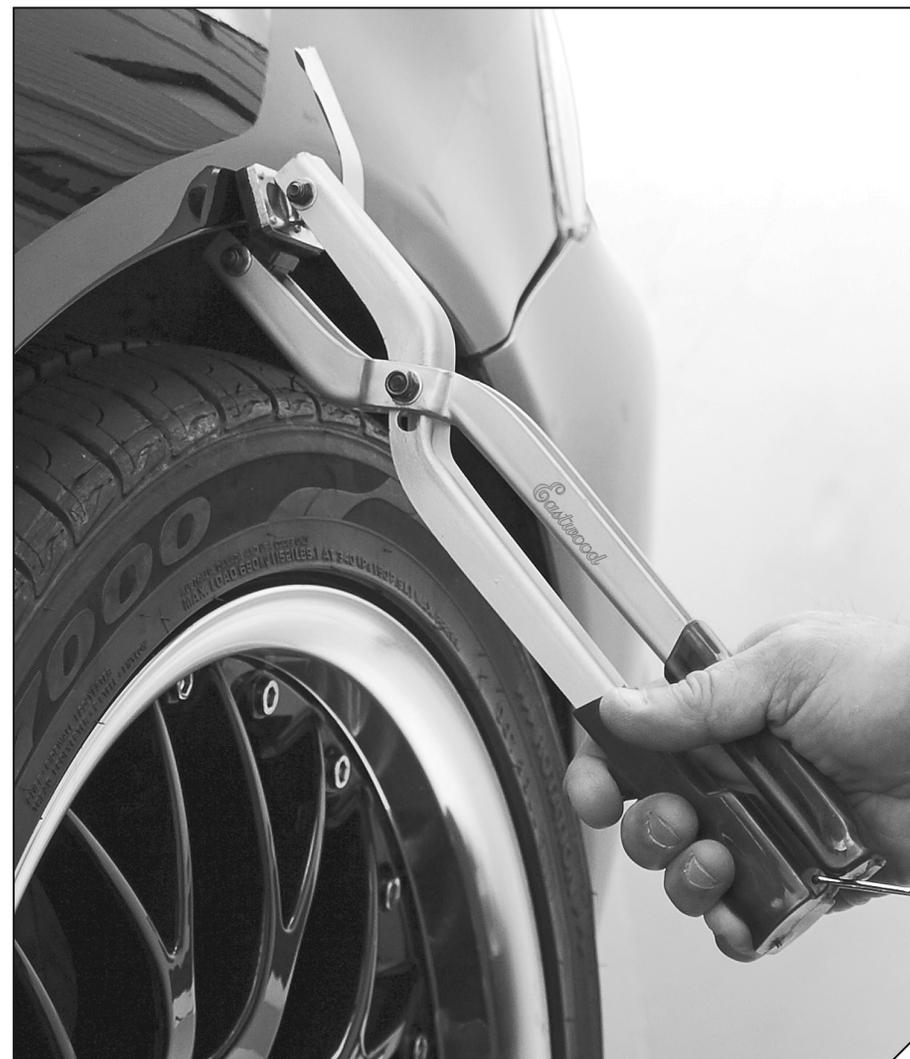
The **EASTWOOD FENDER FINISHER** is a precision engineered tool designed for use by the seasoned professional or the hobbyist. It was created to provide additional fender-lip-to-tire clearance on lowered cars and trucks or those fitted with oversize wheels and tires without the need to remove the wheels from the vehicle.
