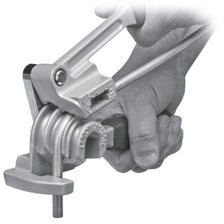
Your Eastwood 180° Tubing Bender is a high quality, precision tool capable of creating accurate, smooth, kink-free bends up 180°. Form lines for brake, transmission, fuel and other automotive applications in annealed aluminum, steel, stainless steel and copper tubing, in sizes from 3/16" to 3/8", left and right handed.
