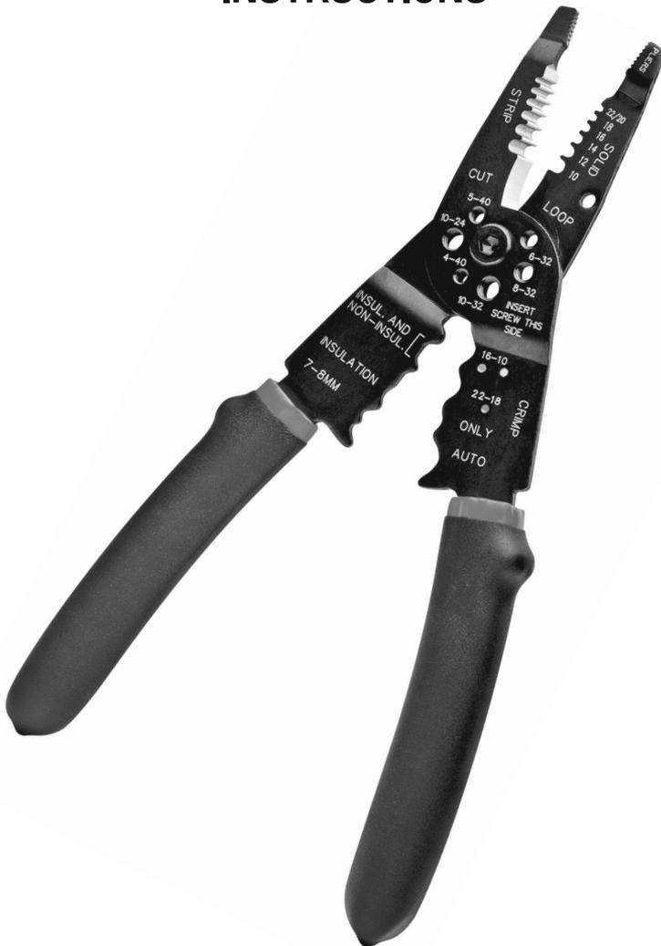
The **Eastwood Precision Wire Stripper, Crimper and Cutter Tool** allows quick, convenient, and accurate one-handed cutting, stripping and crimping of automotive type wire and connectors from 22 to 10 gauges. Also cleanly crimps 7 and 8 mm spark plug wire terminal sizes and cuts #4 through #10 screws.
