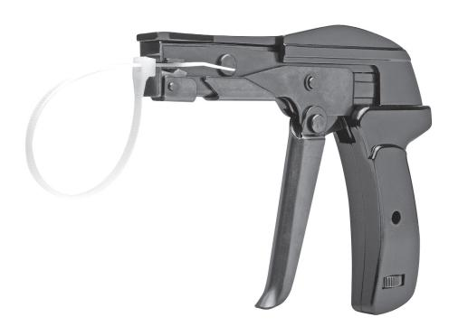
The **Eastwood Professional Cable Tie Gun** allows quick, convenient, one-handed tightening and cutting of cable ties up to 1/4" wide. Just set the tension, grip cable tie end, pull trigger, cut and you are done. Cuts off excess cable tie cleanly with no sharp edges.
