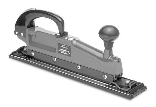
Your **Eastwood Straight-Line Sander** is a heavy-duty professional quality tool ruggedly designed for many years of reliable service. It features a high-efficiency; double-ended, 2 cylinder motor with a positive, double rack and pinion drive assembly for smooth operation and long life. Speed is easily controlled with an infinitely progressive throttled speed control.
