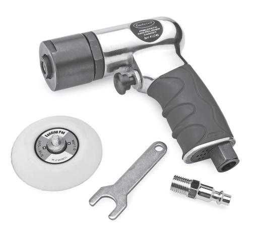
The **EASTWOOD 3" MINI-POLISHER/SANDER** is a compact, lightweight yet powerful tool designed for many years of reliable service. It features a high-torque,4 vane, ball bearing motor and a hardened planetary gearset for long life. Speed is easily controlled with an infinitely progressive throttled trigger control.
