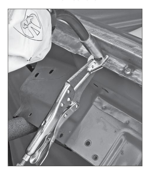
Spot Welding in the past had primarily been done by large resistance welders but can now be achieved with your MIG welder and this **Spot Welding Kit** from Eastwood. Spot welding is accomplished by clamping two panels together and fusing them with a number of welds sequentially-placed rather than a continuous bead to hold the panels together. This kit is designed to be used with Tweco® Style MIG torches.
