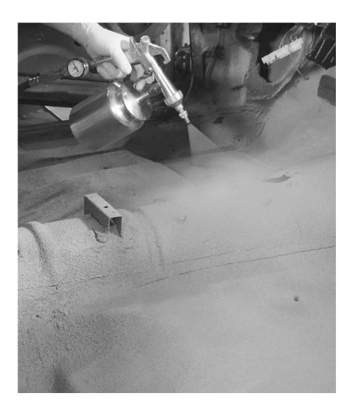
Using advanced ceramic particle technology, the **Eastwood Heat & Sound Barrier Coating** combines excellent heat resistance and sound absorption properties. In addition to offering heat transfer reductions up to  $20^{\circ}$  F [ $6.6^{\circ}$  C] @  $160^{\circ}$  F [ $71.1^{\circ}$  C] &  $600^{\circ}$  F [ $315^{\circ}$  C] high-heat resistance, it will lower decibel readings as much as 5db at a recommended thickness. **COVERAGE**: 1.5 gallons covers 30 sg ft at 60 MIL thickness.
