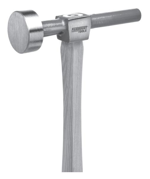
The **FAIRMOUNT™ GRIND YOUR OWN HAMMER** is a high quality forging specifically designed with a generous amount of material in the striking face and back end providing experienced auto body technicians the means to grind their own hammer profiles for personal preferences and to accommodate unusual or seldom encountered metal shapes without resorting to ruining an expensive body hammer.
