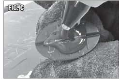
Immediately apply the face of the Pull Button to the previously outlined area and hold firmly in place for 10 to 15 seconds.
