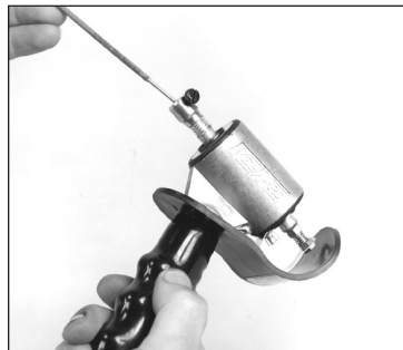
Setup begins by inserting an electrode into the Stitch Welder's brass collar, and snug up the set screw.
