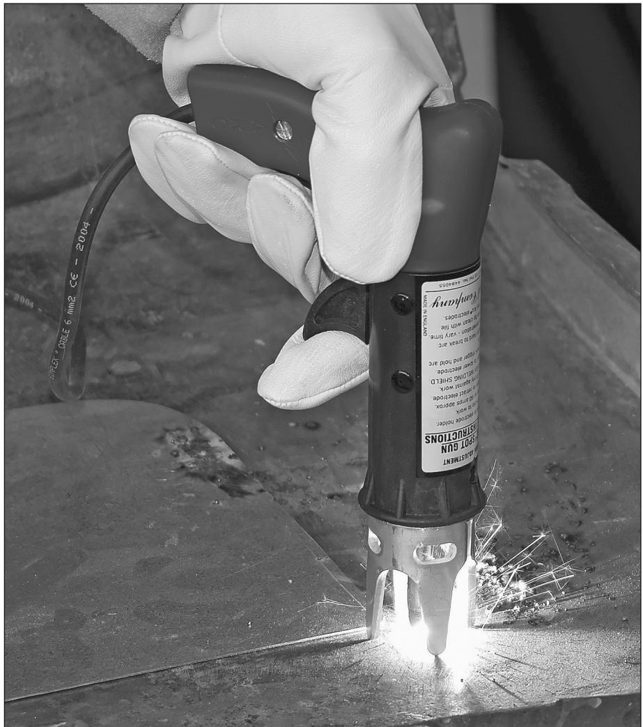
**THE EASTWOOD SPOT WELD GUN** welds two overlapping steel panels (up to 18 gauge) together using an electric arc to melt the top panel, fusing it to the bottom panel. The two panels must be cleaned of all rust, paint, grease, or other material, and must fit tightly together – this is critical to both the strength of the weld and achieving satisfactory results.
