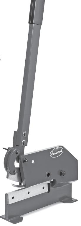
Your **EASTWOOD 8**" **BENCH SHEAR** for metal cutting is designed for quickly and cleanly cutting mild steel, aluminum and other metals. Torque-amplifying, compound linkage provides low effort and a hardened steel ferrule in the Body, with mating Shear hole in the Blade, allow precision shearing of rod material.
