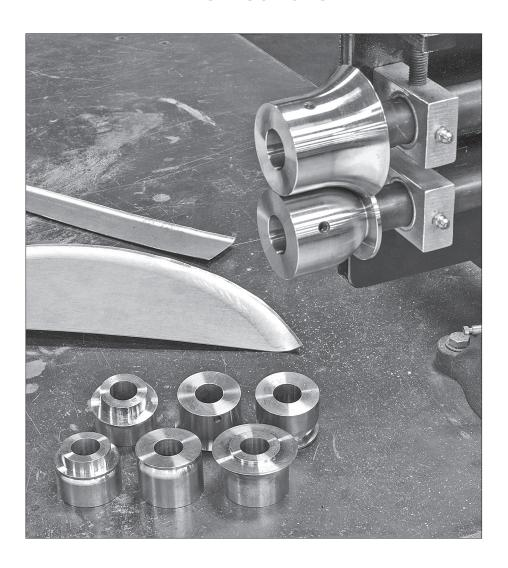
The **EASTWOOD RADIUS EDGE DIES** produce smooth, even, large-radiused edges in steel and aluminum. Fits Eastwood #21487, #32044, 28187, and #21327 Bead Rollers and other units with 22mm shafts.
