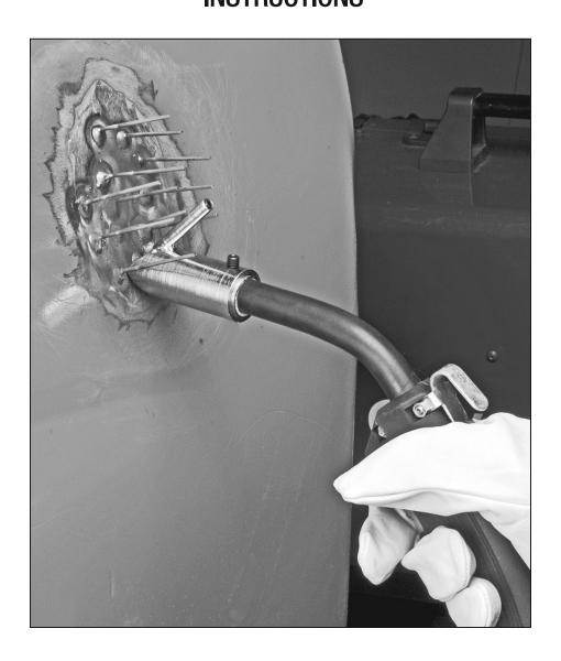
The **EASTWOOD MIG STUD WELDING KIT** transforms your MIG welder into a Stud Welder which can be used to repair and remove dents from sheet metal.
