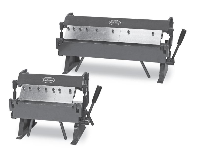
The **EASTWOOD 12" & 24" PAN AND BOX BRAKES** are precision engineered metal working tools designed to produce accurate, variable length bends in angles up to 135° in mild, 20 gauge sheet steel and 18 gauge aluminum in widths up to 12" for the 20664 and 24" for 20665". Create complex shapes such as floor reinforcement channels and ribs, sections of corrugated pickup bed floors; truck bedside panels, inner fender structures and much more, all with one convenient bench-mounted tool.
