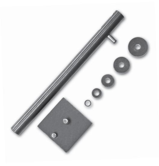
The **EASTWOOD ROD FORMING TOOL** is a high quality, industrial style tool capable of generating a powerful leveraged force to create  $180^{\circ}$  or greater repeatable bends in mild steel and aluminum rods up to  $3/8^{\circ}$  diameter and flat stock up to  $1/2^{\circ}$  wide and  $3/16^{\circ}$  thick.
