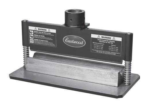
The **EASTWOOD PRESS BRAKE ATTACHMENT** is a precision engineered metal working tool designed to produce accurate, variable length bends in angles up to 90°, in mild steel and aluminum, in widths up to 12" [305mm] and thicknesses up to 3/8" [10mm]. Create complex shapes, such as floor reinforcement channels and ribs, sections of corrugated pickup bed floors, truck bedside panels, inner fender structures, suspension brackets, engine/transmission mounts and much more.
