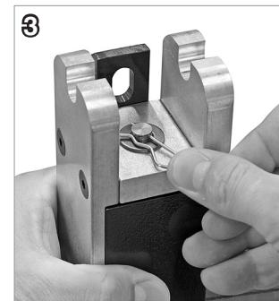
6. Replace the washer and hairpin clip removed in step 3 (Fig 3).
