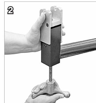
5. Place a washer (removed in step 3.) over the turned end of the jackscrew shaft. Slide the long threaded bushing with the jackscrew and handle up into the lower square block of the Frame with the machined groove facing outward and over the set screw in the lower block. Tighten the set screw.
