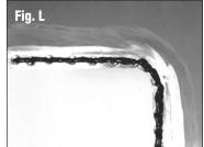
Begin riveting (using 1/8" flush rivets) at a corner or radius first to keep panel flush. Continue installing rivets working evenly from the start point until all rivets are set. Now use a spreader to smooth the adhesive. The entire flange area and seam are protected against rust with the adhesive, on both sides of repair (FigS M-N).
