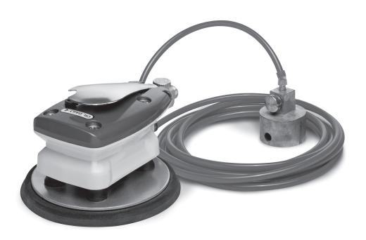
The **5" WET JITTERBUG SANDER** is a heavy-duty professional quality tool designed for many years of reliable service. It features a high-efficiency sealed ball bearing drive assembly for smooth, low vibration operation and long life. The precision diecast housing provides a solid foundation and offers ergonomic, one handed operation with speed controlled by an infinitely variable hand paddle and rotary knob speed limiting control.
