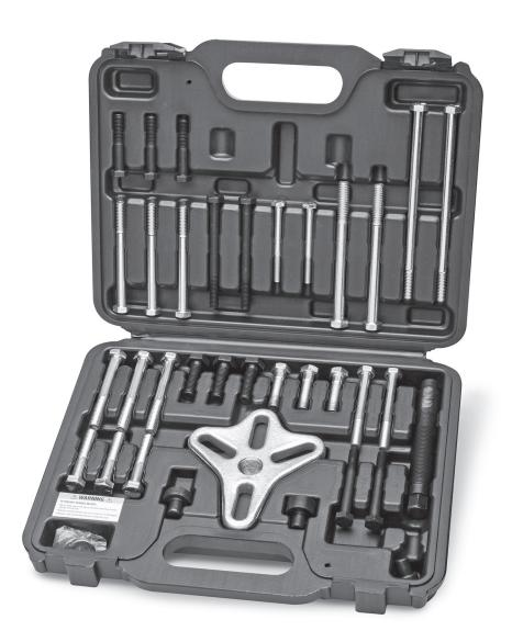
The **ROCKWOOD HARMONIC BALANCER PULLER** provides a means to safely pull most automotive engine Harmonic Balancers without damage to valuable components. The forged steel Yoke offers a range of 2 and 3 bolt patterns from 1.75" to 3.75" (44mm to 95mm) bolt circles.
