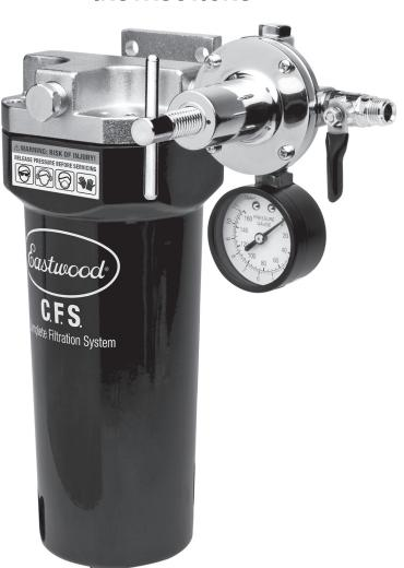
The **EASTWOOD C.F.S.** (Complete Filtration System) includes a high-capacity canister with a long-life 1-micron coalescing filter, and petcock drain to trap moisture and other impurities from a compressed air supply. The Regulator features a 0 to 160 PSI Gauge. It also features an integral mounting bracket for secure mounting and can be easily upgraded to air drying capability with the optional DeVilbiss® #130524 Desiccant Kit (Eastwood item #51567).
