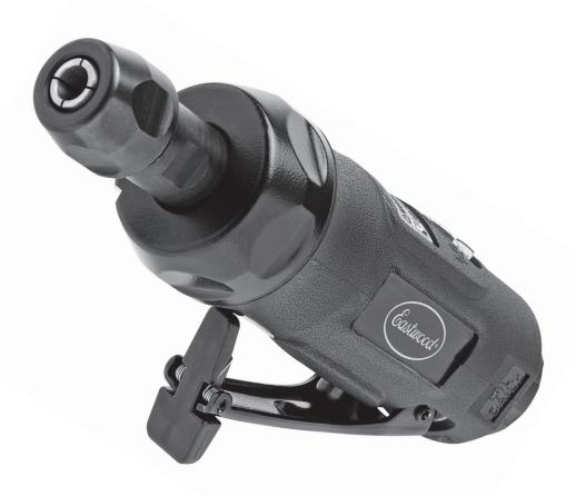
The **EASTWOOD 1/4"** AIR **DIE GRINDER** features a contemporary rubber covered, aluminum body for light weight and minimal vibration. The positive 1/4", non-slip collet allows quick, convenient and secure accessory changes. A high-performance, 4 vane, ball bearing motor provides smooth operation and long life. Speed is easily controlled with an infinitely progressive throttled paddle type control.
