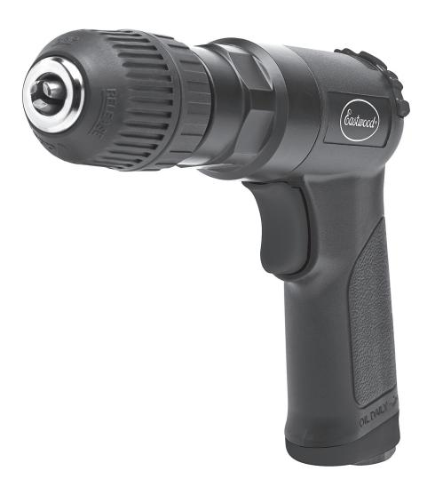
The **EASTWOOD 3/8" COMPOSITE DRILL** is constructed with a rugged and lightweight composite housing. It features a convenient Keyless Chuck, positive-locking forward/reverse control, a high-performance, 5-vane, ball bearing air motor, and hardened planetary gear set for smooth operation and long life. Speed is easily controlled with an infinitely progressive throttled trigger control.
