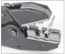
Place the stripped end of the wire into the smaller "U" feature of the Connector with the Silicone Connector Wire Seal nested in the larger "U" (FIG 5).
