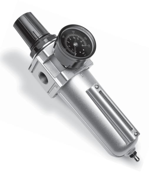
The **ROCKWOOD 1/2" NPT AIR FILTER/REGULATOR** includes a high-capacity, drainable Coalescing Filter and Bowl to trap moisture and other impurities from a compressed air supply. The Regulator features a 0 to 230 PSI Gauge. Also included is an integral mounting bracket for secure mounting.
