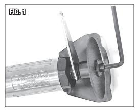
• Place replacement wheel over the stepped 3/8" [9.5mm] diameter portion of the shaft, replace Retaining Washer in the proper bevel-out position then use the wrenches to tighten (FIG 1).
