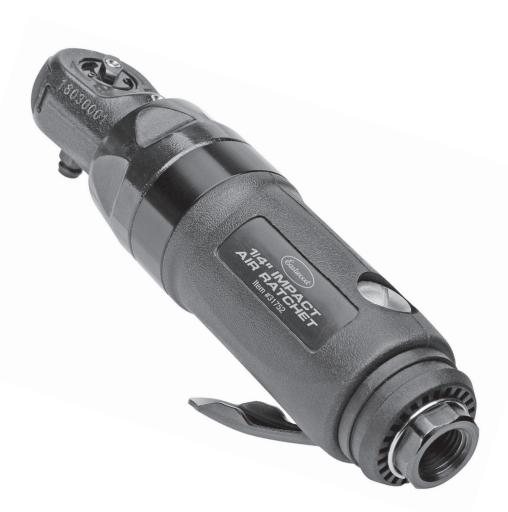
The **EASTWOOD 1/4" IMPACT AIR RATCHET** offers high performance in a compact, soft-grip, lightweight aluminum housing that fits in the tightest areas. It features a powerful, four-vane, ball bearing motor with an efficient twin-hammer drive. Includes forward and reverse with an infinitely variable throttle control.
