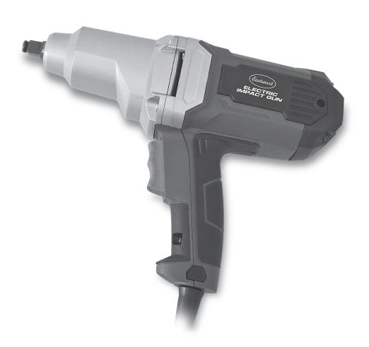
The **EASTWOOD 1/2" ELECTRIC IMPACT WRENCH** is great for use where a compressed air supply is unavailable. The powerful 7.5 Amp motor and 1/2" square drive powers impact sockets and accessories with ease. A simple, Reverse/Forward rocker switch provides instant response. Features a "plugged—in" indicator lamp for safety and convenience.
