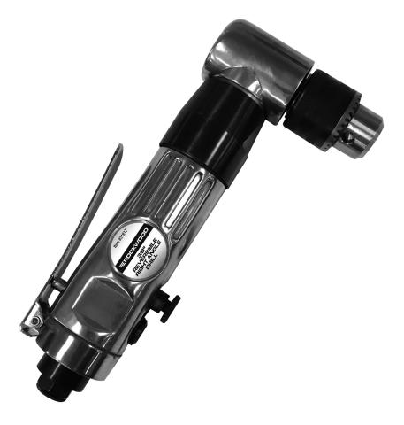
**YOUR ROCKWOOD 3/8" REVERSIBLE RIGHT ANGLE DRILL** is a heavy-duty professional quality tool with hardened bevel and planetary gears ruggedly designed for many years of reliable service. It features a positive-locking forward/reverse control. A high-torque, 5-vane, ball bearing air motor provides smooth operation and long life. Speed is easily controlled with an infinitely progressive trigger control.
