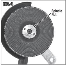
• While holding the Spindle with the Arbor Wrench, set the pins of the Spindle Nut Spanner into the holes of the Spindle Nut and tighten it securely (FIG 4).
