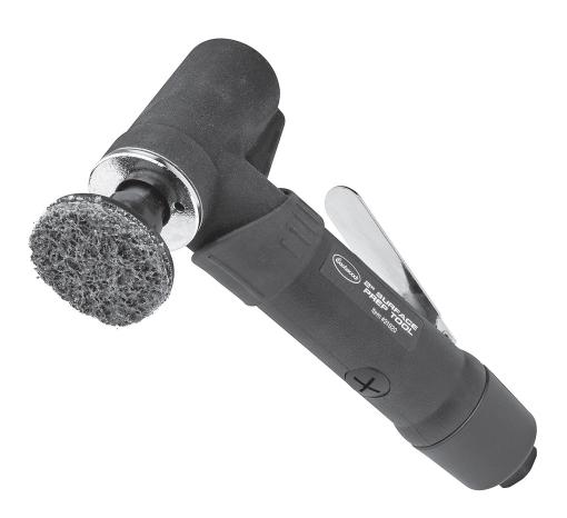
The **EASTWOOD 2" SURFACE PREP TOOL** is a heavy-duty professional quality tool ruggedly designed for many years of reliable service. It features a strong, lightweight composite housing for comfort and durability. A high-torque, 5-vane, ball bearing air motor provide smooth operation and long life. Speed is easily controlled with an infinitely progressive trigger control.
