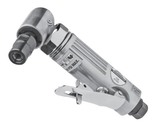
The **Rockwood Right Angle Air Die Grinder** is a heavy-duty professional quality tool ruggedly designed for many years of reliable service. It features positive 1/8" & 1/4", non-slip collets for quick, convenient and secure accessory changes. A high-torque, 4 vane, ball bearing motor with hardened bevel gears provide smooth operation and long life. Speed is easily controlled with an infinitely progressive trigger control.
