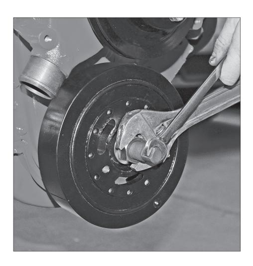
**THE EASTWOOD HARMONIC BALANCER INSTALLER SET** provides a means to safely install most automotive engine Harmonic Balancers and pulleys without damage to balancers or crankshaft ends. A selection of 13 most popular thread size studs fits most automotive crankshafts with internal threaded ends. The large 1-5/8" diameter bearing provides a large surface area to evenly draw in balancers.
