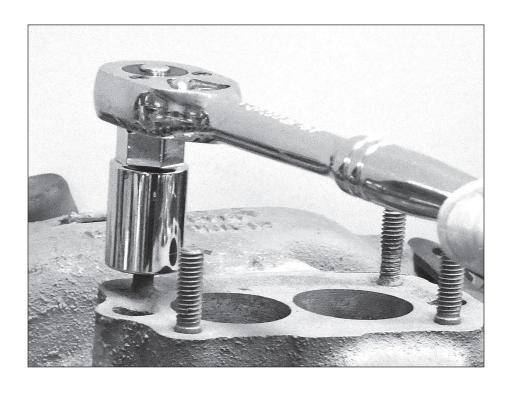
**THE EASTWOOD STUD REMOVER/INSTALLER SET** allows positive, damage free removal and installation of threaded studs providing grip by solidly surrounding them with three hardened steel cylinders.
