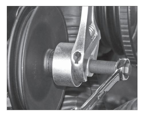
**THE EASTWOOD POWER STEERING PULLEY REMOVER/INSTALLER** allows damage-free removal and reinstallation of most friction fit pulleys found on power steering pumps and many other belt driven automotive and industrial devices. This tool is constructed of high-strength steel components, designed for frequent, heavy duty use and will provide years of reliable service.
