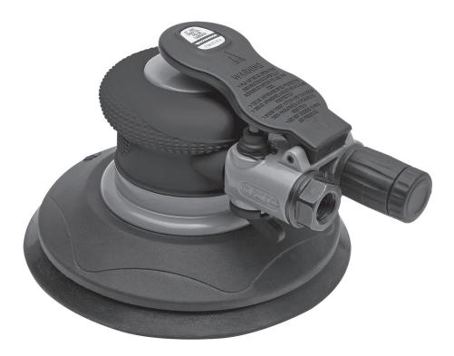
The **ROCKWOOD 6**" **AIR ORBITAL PALM SANDER** is a powerful, high-speed sander designed for high-efficiency. It features a sealed ball bearing drive assembly for smooth, low vibration operation and long life. The precision diecast housing provides a solid foundation and offers ergonomic, one handed operation with speed controlled by an infinitely variable hand paddle and thumb lever speed limiting control.
