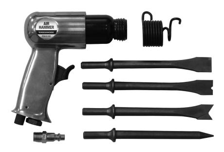
The **ROCKWOOD AIR HAMMER & CHISEL SET** features a high-performance 4500 bpm (blows per minute) design for quick and efficient operation. It accepts any standard 0.401" Parker Taper shank air hammer tool bit and includes four of the most popular tool bit configurations.
