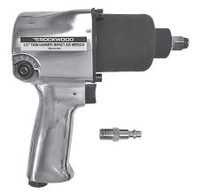
Reversible, variable speed, 6 vane, ball bearing air motor, twin-hammer impact drive Side mounted torque limiting control knob. 0 lowest, 5 highest
