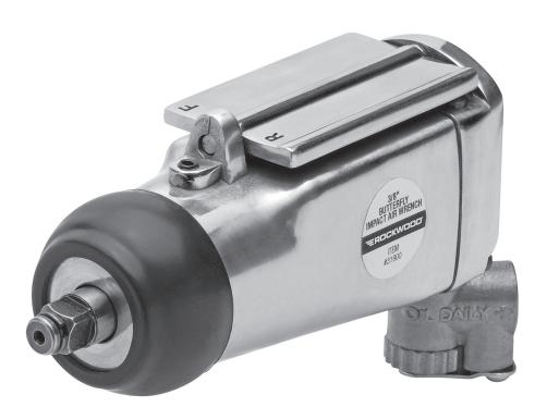
The **ROCKWOOD 3/8" "BUTTERFLY" IMPACT AIR WRENCH** features a large-capacity five-vane, ball bearing motor with a twin-headed hammer dog. Fully reversible with an infinitely throttled "Butterfly" type paddle control.
