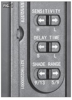
**To Adjust Sensitivity:** Slide Sensitivity Switch to the High "H" position to increase sensitivity for low amperage welding. Slide Sensitivity Switch to the Low "L" position when welding in sunlight or bright ambient light.
