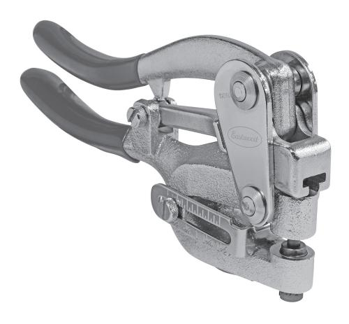
The **EASTWOOD 14 GAUGE METAL HAND PUNCH** is designed to rapidly produce repeatable, clean, accurate holes in mild steel up to 14 Gauge (5/64") [2mm] thick making it perfect for creating rivet holes for custom fabrication work. A compound-leverage design greatly amplifies hand pressure providing greater accuracy, speed and convenience. The 16 Piece, Eastwood Metal Hand Punch is supplied with 7 Male and Female Die Sets and Die Installation Tool.
