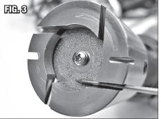
• To begin grinding, allow several seconds for the motor to reach full speed then gently place the tungsten into the proper width slot (FIG 3).
