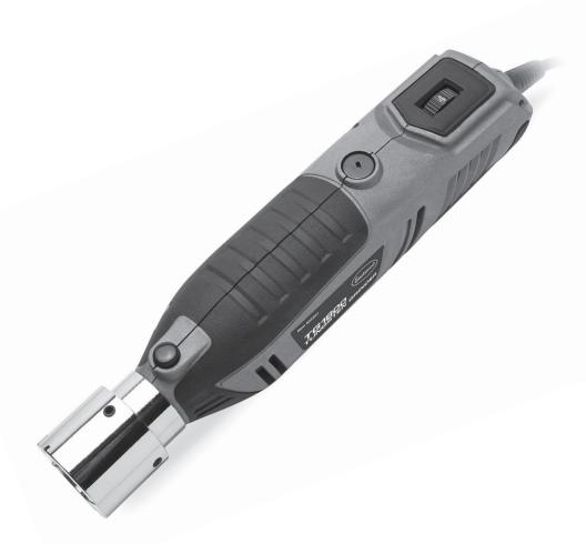
This **EASTWOOD TG1800 TUNGSTEN GRINDER** features a long-lasting, double-sided, Diamond Grinding wheel capable of providing over 200 tungsten sharpening's before requiring replacement. The high-speed electric motor allows the user to produce a finely sharpened point in the ideal 10° or 22.5° preferred angle within seconds. The uniquely designed tungsten guide accepts both 1/16" and 3/32" diameter tungsten electrodes for both breaking deformed tips and prepping new tungsten rods.
