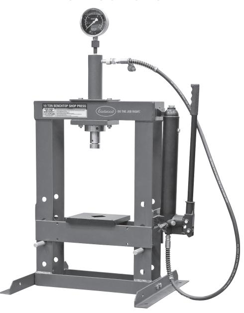
The **EASTWOOD 10 TON HYDRAULIC BENCH PRESS** is excellent for many mechanical procedures requiring a strong linear pressing force for disassembly or assembly operations. A generous 6.88" Ram Stroke and adjustable 4.3 to 14.3" vertical working range can easily accommodate many ball joint, u-joint, bearing, bushing and gear pressing projects.
