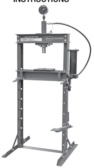
The **EASTWOOD 12 TON FLOOR SHOP PRESS** is excellent for many mechanical procedures requiring a strong linear pressing force for disassembly or assembly operations. A generous 7.1" Ram Stroke and adjustable 3" to 36" vertical working range can easily accommodate many ball joint, u-joint, bearing, bushing and gear pressing projects. The convenient Foot Pedal feature provides a choice of hands-free, foot actuated operation or the standard, hand operation pump function.
