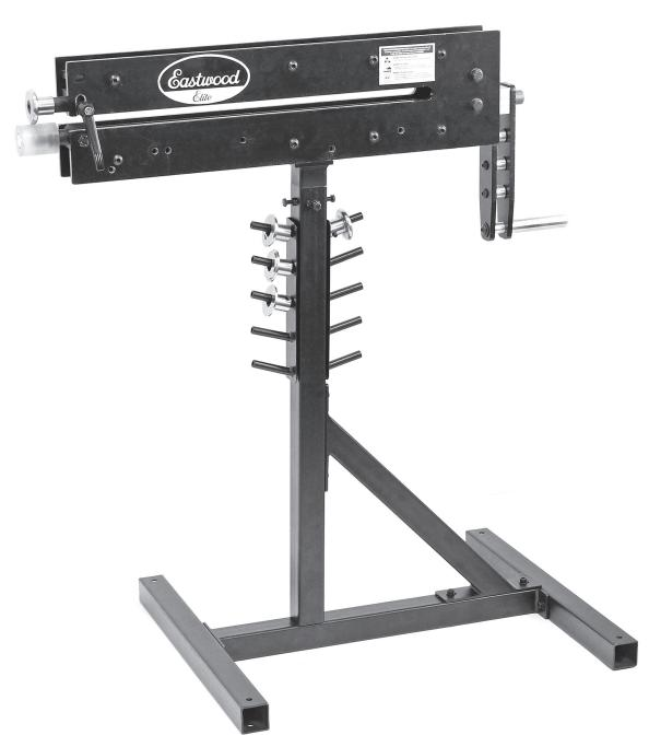
The **EASTWOOD BEAD ROLLER STAND** is designed to fit the Eastwood #32044, 19" Bead Roller (not included), and allows a full 360° field of swivel rotation. Avoid chasing the work, rotate the Bead Roller to the position most comfortable for increased precision and easier operation.
